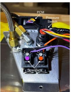
Take your wiring harness and plug in the pressure switch connector until you hear it click. Plug in the solenoid connectors. The connector with the purple wire will plug in directly behind the 90\* fitting. Plug in the other solenoid connector. Each of those connectors has a small allen screw to secure the connector. Tighten those but **DO NOT OVER TIGHTEN.**
