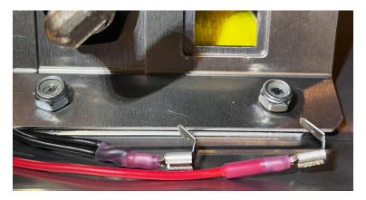
Take the black wire and cut the ring terminal off. Do this as close to the ring terminal as possible. Strip the wires and insert & crimp the supplied piggyback spade connector.
