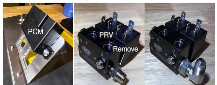
Slide the PRV under the bracket as shown. <u>NOTE - The PRV does not mount in the same fashion as described in the ARB instructions</u>. Install the second 90\* BSP fitting into the port on the PRV as shown. Install the pressure sensor in the port as shown.
